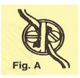
through from rear, strip leads <sup>1</sup>/4" and connect to switch terminals as shown in Fig. A. Pull wires from rear to remove slack and insert switch in hole. Secure switch assembly with screw nails supplied.
