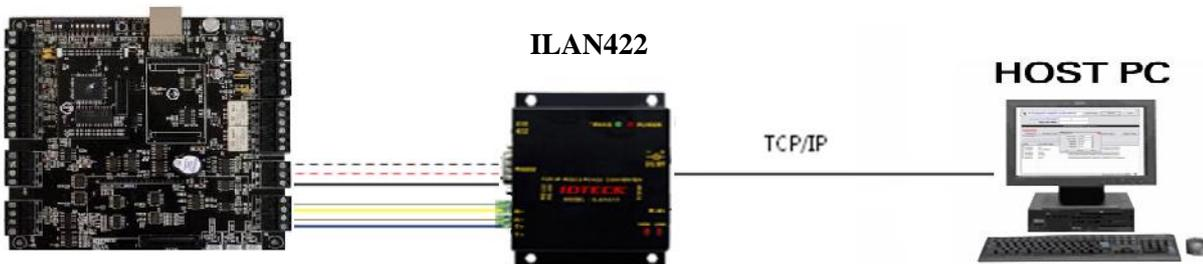
Figure: TCP/IP Converter between Host PC and iCON100
