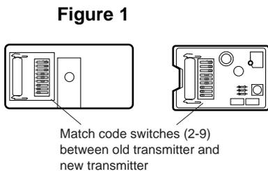
Place the new transmitter and the original transmitter side by side as shown (Figure 1) and set the switches in both transmitters to matching positions (+,0,-). Use a pen or screwdriver to slide the code switches.
